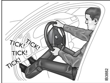
*Braking with ABS brakes.
